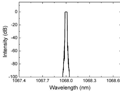
Fig. 5. Simulated spectrum, with a 0.03-nm FWHM bandwidth.
