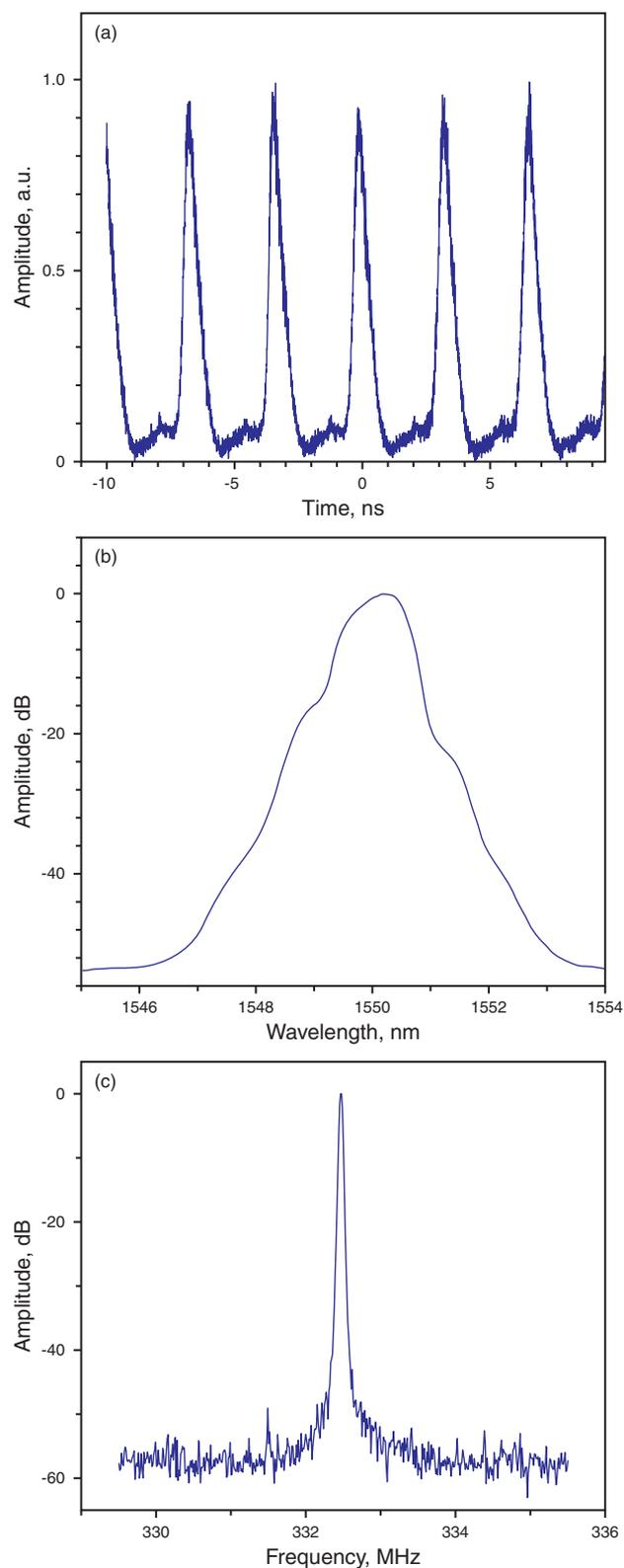
**Figure 3** (online color at [www.lphys.org](http://www.lphys.org)) (a) – oscilloscope temporal trace of the high harmonic mode-locked 600 ps pulses from the cavity with spectral filtering and with 200 m of non-linear fiber, (b) – optical spectrum, and (c) – RF trace
