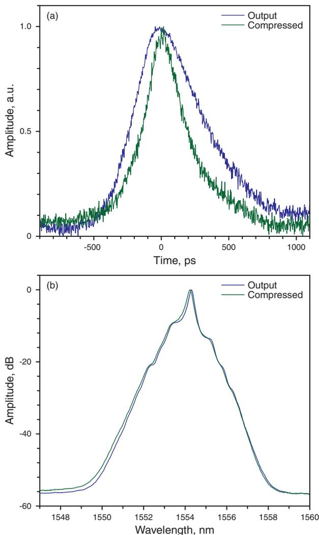
**Figure 5** (online color at [www.lphys.org](http://www.lphys.org)) (a) – oscilloscope trace of output 600 ps pulses, from high harmonic mode-locked cavity with 400 m of non-linear fiber, to 350 ps in 21 km of STF and (b) – the optical spectrum before and after compression
