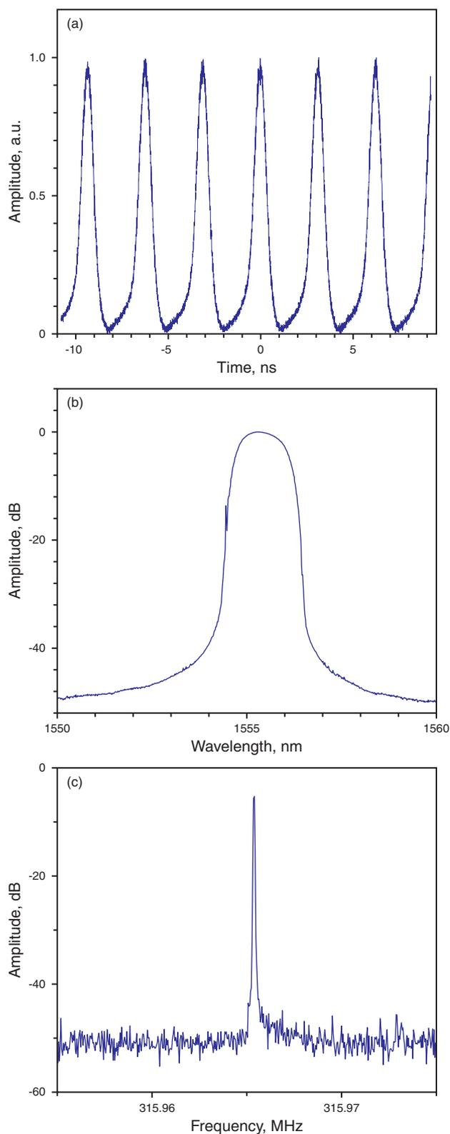
**Figure 2** (online color at [www.lphys.org](http://www.lphys.org)) (a) – oscilloscope temporal trace of the high harmonic mode-locked 750 ps pulses from the cavity without filter and with 100 m of non-linear fiber, (b) – optical spectrum, and (c) – RF trace
