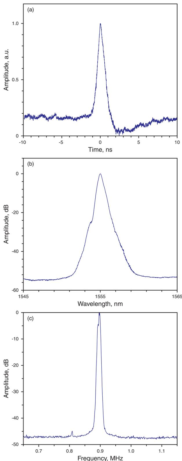
**Figure 4** (online color at [www.lphys.org](http://www.lphys.org)) (a) – oscilloscope trace of the single-pulses mode-locked cavity without filter and with 200 m of non-linear fiber, (b) – optical spectrum, and (c) – RF trace
