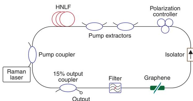
**Figure 1** (online color at [www.lphys.org](http://www.lphys.org)) Raman oscillator configuration. HNLF – highly nonlinear fiber
