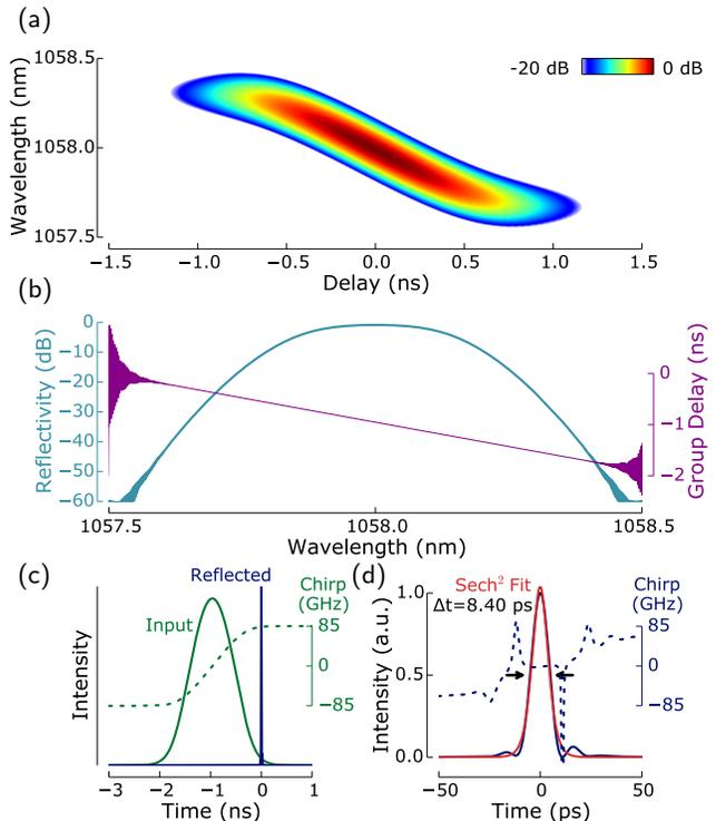
Fig. 2. Numerical modeling results: (a) Giant-chirped pulse spectrogram. (b) CFBG reflectivity and group delay, for CFBG properties:  $n_0 = 1.45$ ,  $\delta n = 5 \times 10^{-5}$ ,  $\frac{d\lambda_B}{dz} = 0.0048$  nm/mm,  $L = 200$  mm and 60 mm FWHM Gaussian apodization envelope. (c) & (d) Incident and reflected pulses from the CFBG, showing pulse compression.
