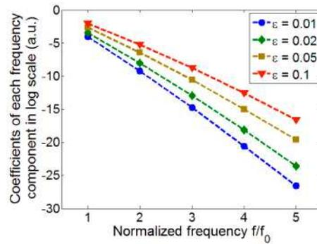
Fig. 6. Coefficients of each frequency component based on Eq. (5) at different modulation depth  $\varepsilon$ . The vertical axis is plotted in logarithm scale. The coefficients show very good linearity which verifies the validity of the exponential decay model we have proposed in Eq. (3).
