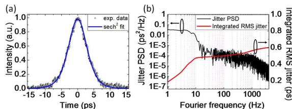
Fig. 4. (Color online) (a) Cross-correlation trace from the two synchronized all-fiber mode-locked lasers. (b) Sum-frequency generation intensity-noise power spectral density (PSD) and integrated timing jitter of the synchronized lasers.
