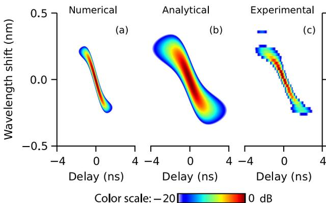
Fig. 1. Spectrograms of the steady-state output pulse at a center wavelength of  $\lambda_c = 1065$  nm. (a) numerical, (b) analytical and (c) experimental after [9].
