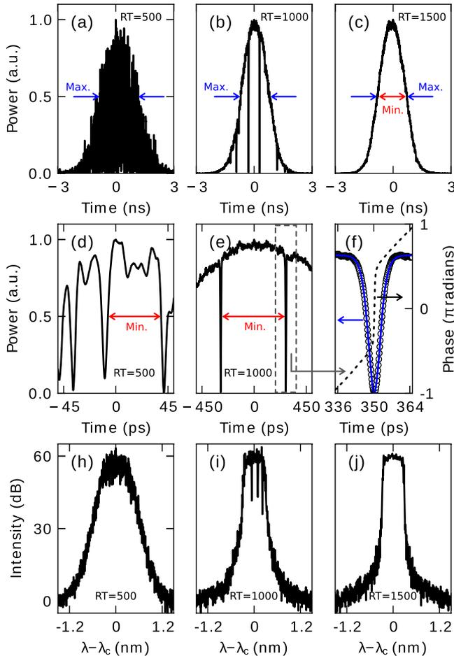
Fig. 2. Temporal [top, (a)–(c)], zoomed temporal [middle, (d), (e)], phase (f), and spectral [bottom, (h)–(j)] profiles for three different stages of the characteristic pulse evolution within the oscillator cavity. RT, round-trip number; min, internal pulse width; max, envelope duration. Center wavelength  $\lambda_c = 1065$  nm.
